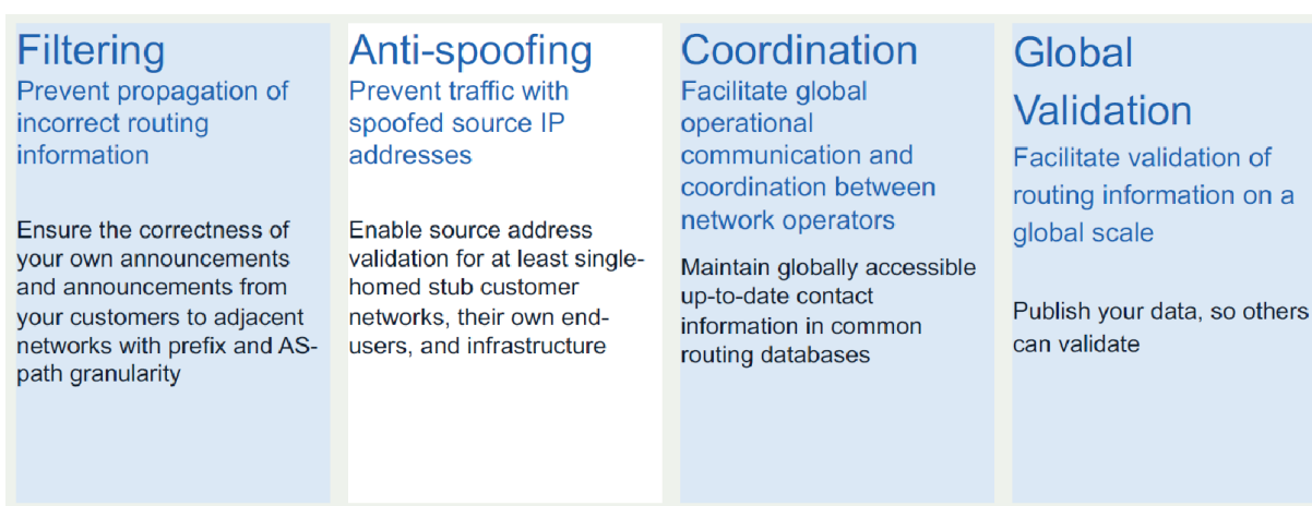
Fig. 3 MANRS Actions for Network Operators (source: MANRS)
